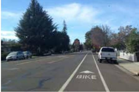
Figure 1-7 A standard bike lane on Cuesta Drive includes painted edges lines, delineating the bike lane from the parking lane
