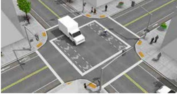
**Figure 4-11 The NACTO Urban Bikeway Design Guide provides design guidance for intersection crossing markings.**
