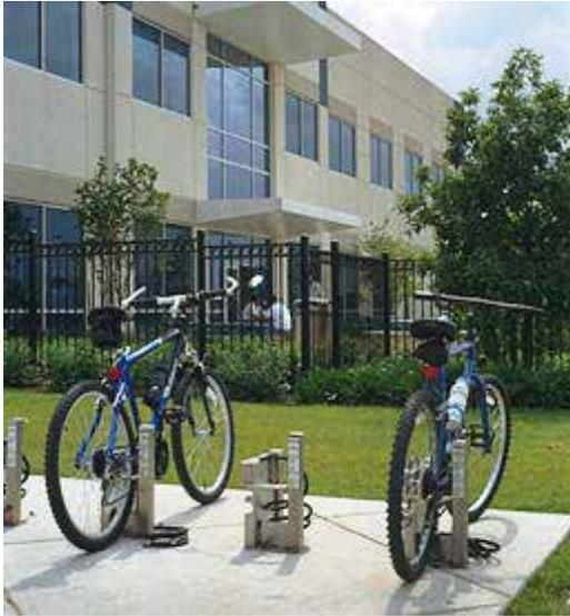
Figure 1-22 Class II “Crankcase” Bicycle Racks
