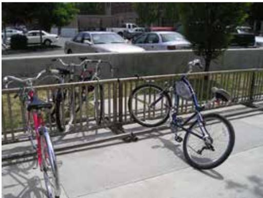
Figure 1-24 The Class III bike parking as defined by the BTG only allows users to lock the wheel of their bike, not the frame. This makes bikes more vulnerable to theft.
