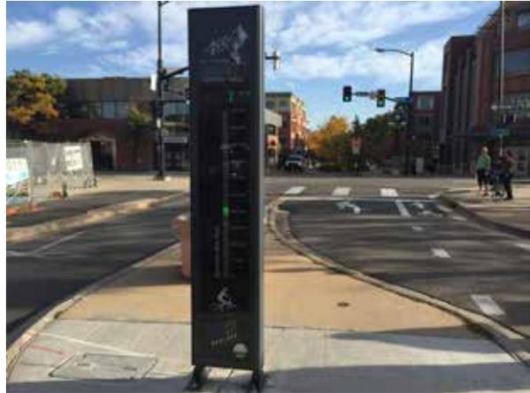
**Figure 4-19 An automatic bike counter in Boulder, Colorado**
