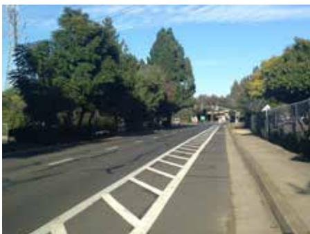
Figure 1-10 A buffered bike lane on Moffett Boulevard separates bikes from adjacent traffic
